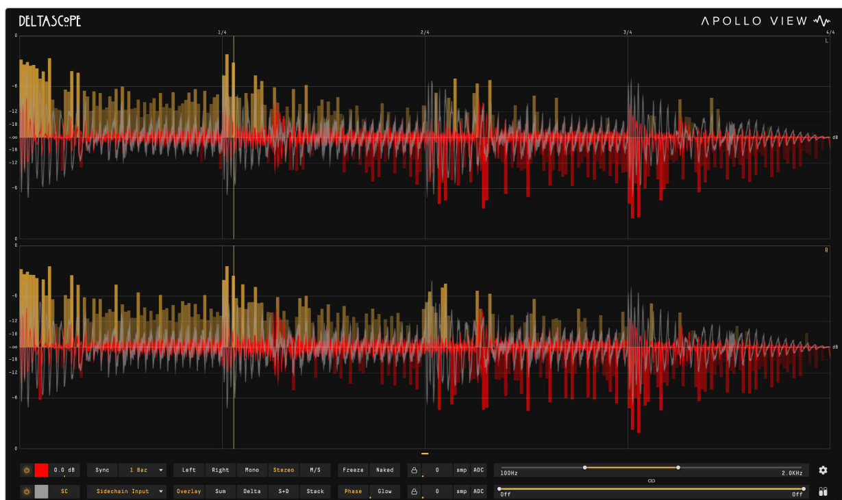
Band at 100 Hz - 2 kHz feeding the phase display: correlation is analysed inside the band only.
