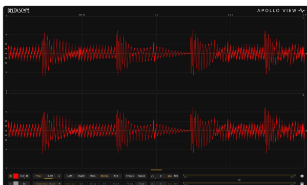
Rolling mode, Free-run at a 2 s window: the newest audio enters at the right edge...
