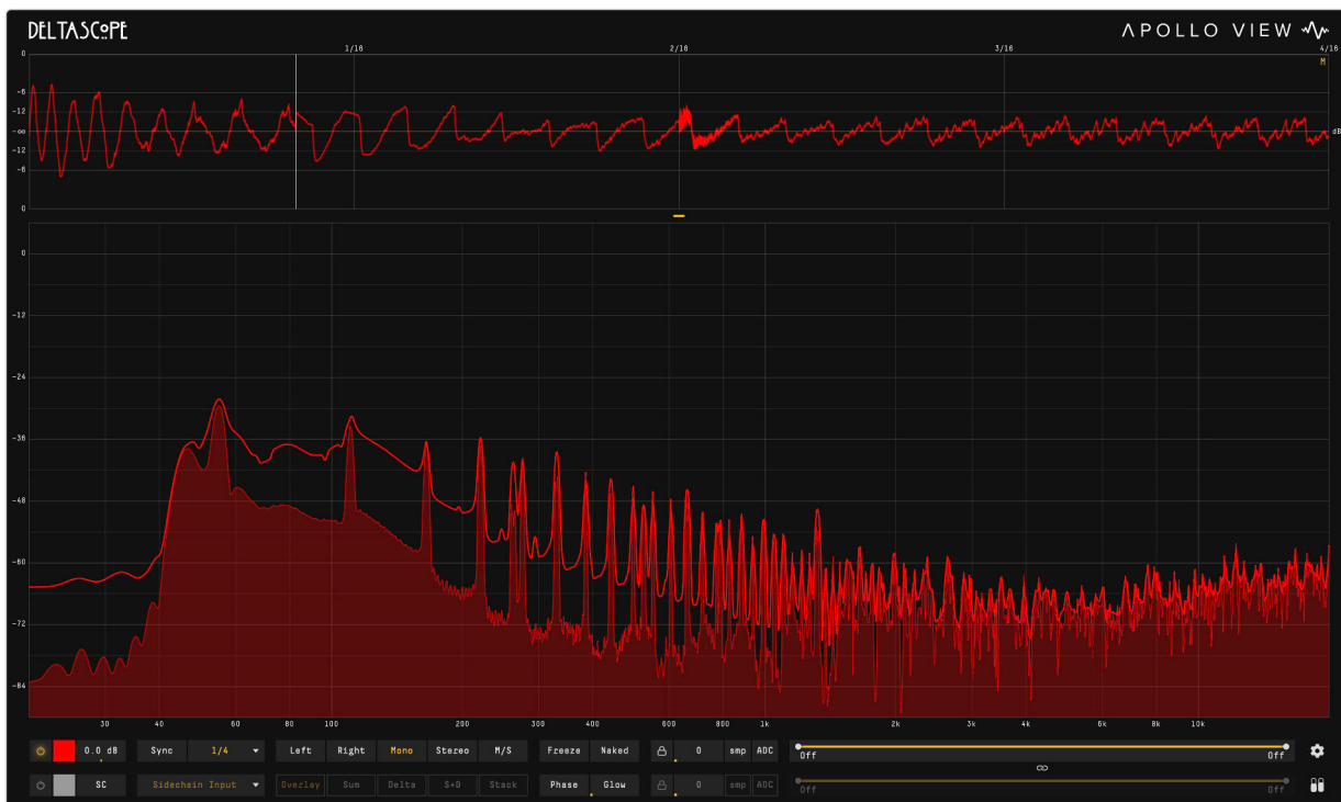
Spectrum pane opened wide (Mono), peak-hold line above the live curve.
