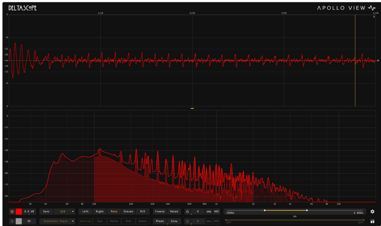
Band at 100 Hz - 2 kHz with Filters » FFT active: the spectrum fill dims outside the band.
